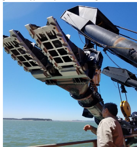
Figure 3. Typical hydraulic dredge head
