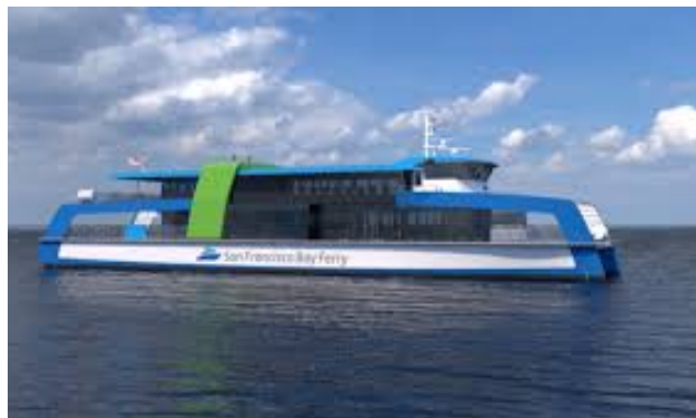
Left: 400-passenger battery-electric ferry to be built for San Francisco Bay Ferry. Specifications are 142ft 1in x 34ft 9in Subchapter K vessels.
