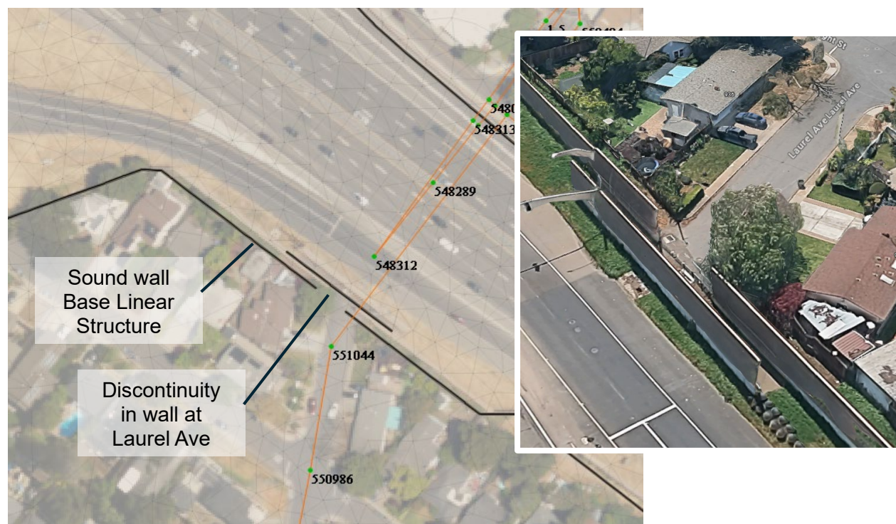
Figure 4-12: Barrier Discontinuity Near Willow Road Interchange
