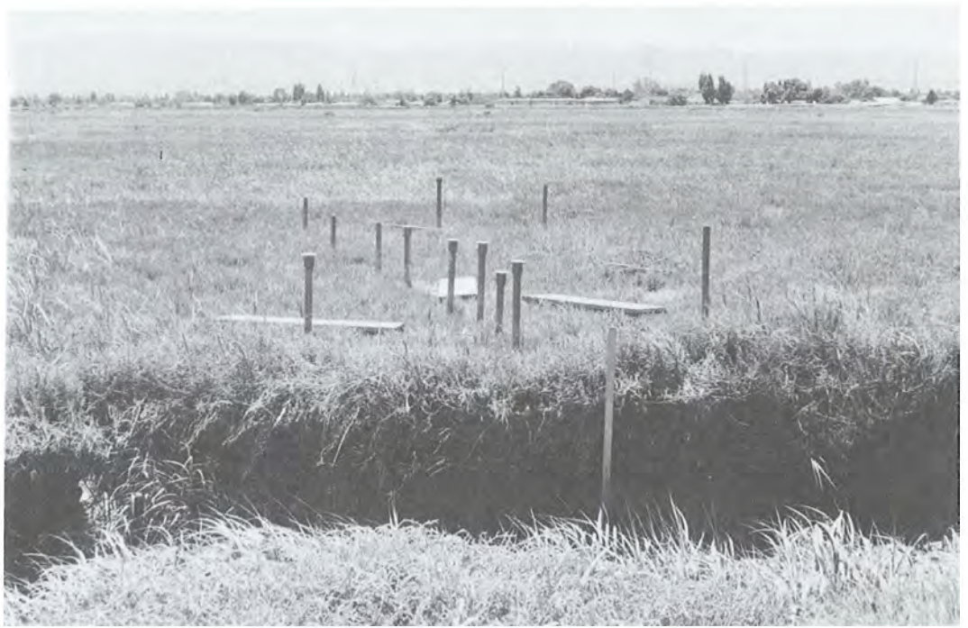
Plate 3. Piezometer set-up in Cooley Landing marsh (looking south). The row from the channel consists of the C piezometers.
