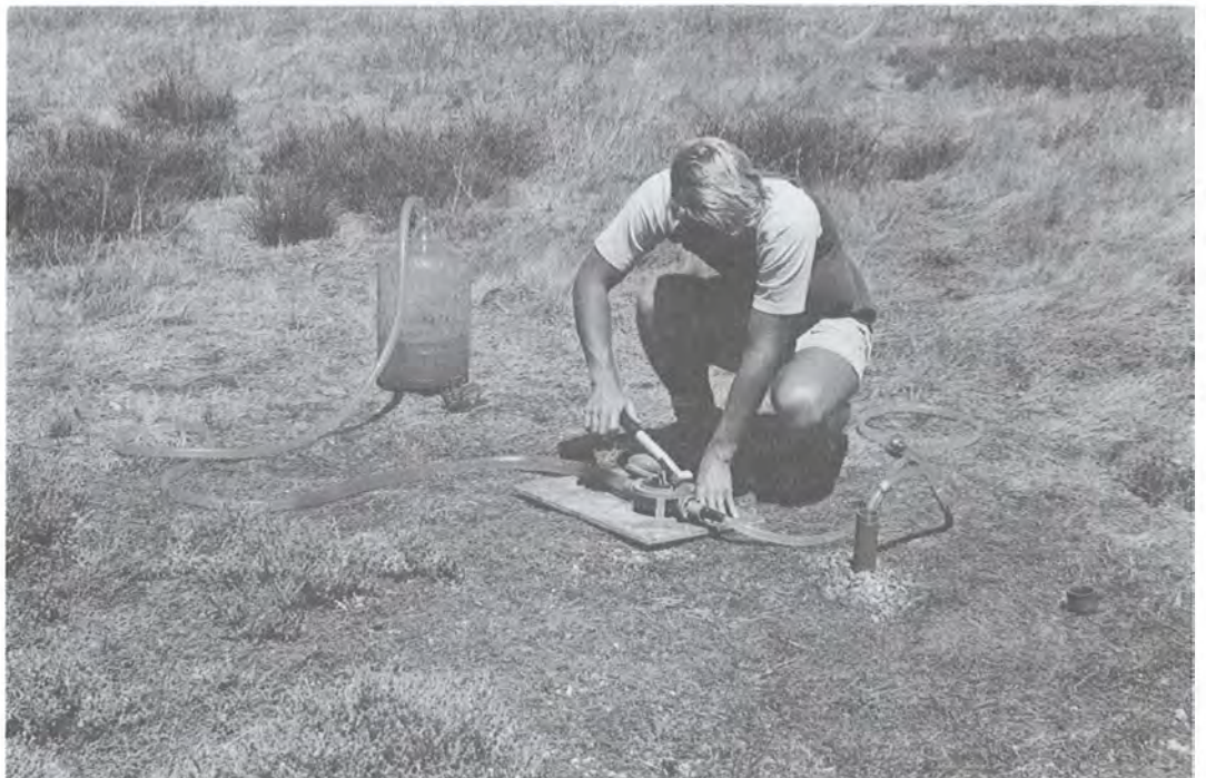
Plate 6. Pumping of a piezometer in the Palo Alto Flood Control Basin. Five gallon bottle for measuring pumped volumes.
