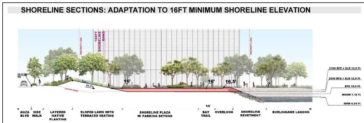
Figure 5: Cross section diagram of shoreline elevations and projected sea level rise through 2100.
